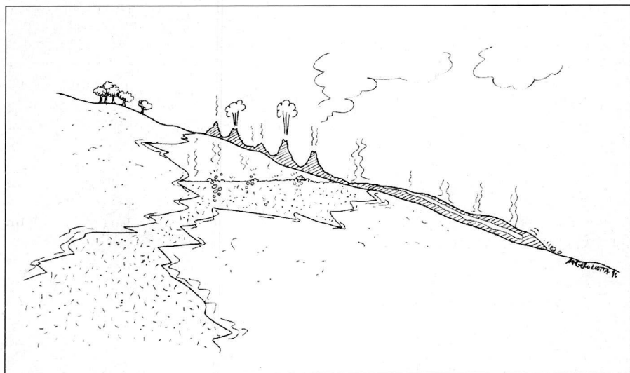
Fig. 2 - Hornitos aligned with the direction of the fissure: at the lower end is placed the effusive vents, named "oven mouth".
